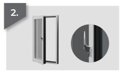
Return window to the closed position before turning the handle 180° to open the window inwards
