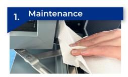
Clean away any dirt or debris from the hinge or pivots, sliding shoe and track
