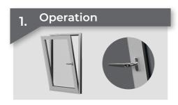
Turn the handle 90° to tilt the window for ventilation
