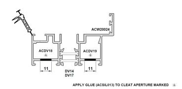
Using the adhesive provided, apply to the inside of the outer-frame section, just passed both the punched out holes. Do this to each end of all the sections of outer-frame.
