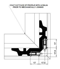
Once the cleats are fully inserted, position the chevron into the alignment slots. Push the joints together. This is best done by fitting the left and right pieces of outer-frame to the bottom section followed by the fitting of the top piece.
